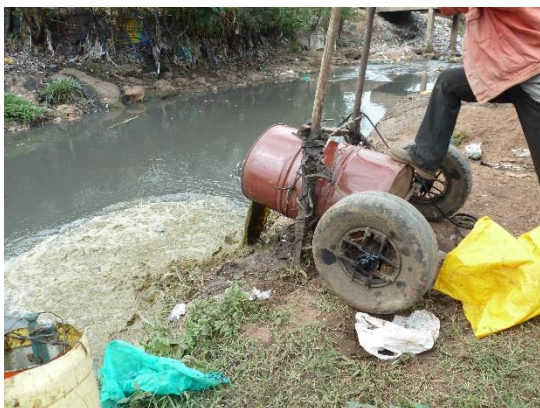
Figure 3 Manual emptier discharging the collected faecal sludge in a nearby stream © GIZ/Doreen Mbalo
