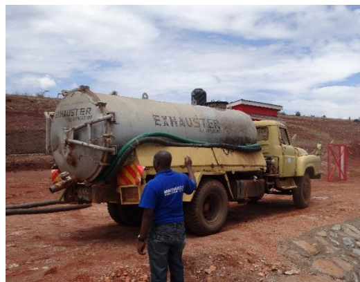
Figure 4 Private vacuum truck at a designated discharge point © GIZ/Alexandra Dubois
