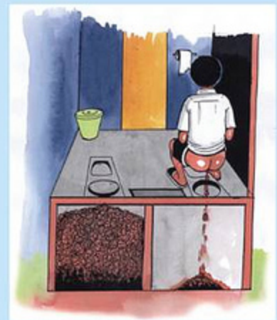
WHEN THE FIRST CHAMBER IS FULL, COVER IT AND BEGIN USING THE SECOND CHAMBER UNTIL IT IS FULL
