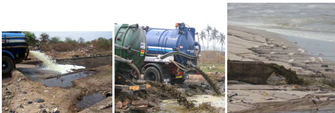
Figure 3.7: Desludging honey trucks at Teschie-Nungua (left) and Lavender Hill (middle and right)
