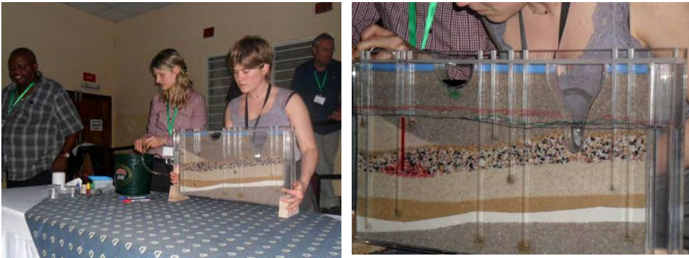
Picture 18+19: Model demonstrating groundwater contamination from an abstraction well (red) and a pit latrine (green).
