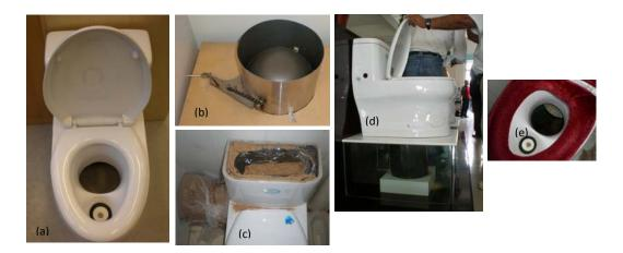
**Figures 3-4a to 3-4d**. The urine-diversion dry (UDD) toilets at EETP. (a) The toilet with the urine hole at the bottom of the picture and the faecal hole in the middle. (b) The turning bowl mechanism. (c) The sawdust dispenser. (d) An EETP model showing the faecal chute connected to the toilet. (e) The third toilet prototype with a sliding plate. [A. Flores, taken in September 2007.]
