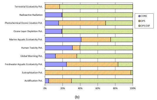
*Figures 5-7a and 7b.* Life Cycle Impacts of the a) DRY and b) WET systems broken down by percentage contributions from construction (CONS), operation (OPS) and system expansion (OPS-EXP).
