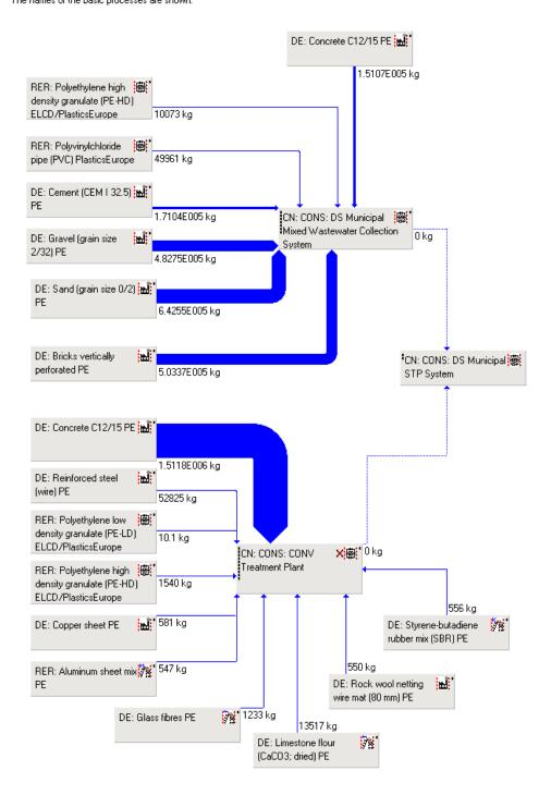
**Figure C-2.** GaBi LCA Plans: Construction of the Conventional Waterbourne System (WET System).
