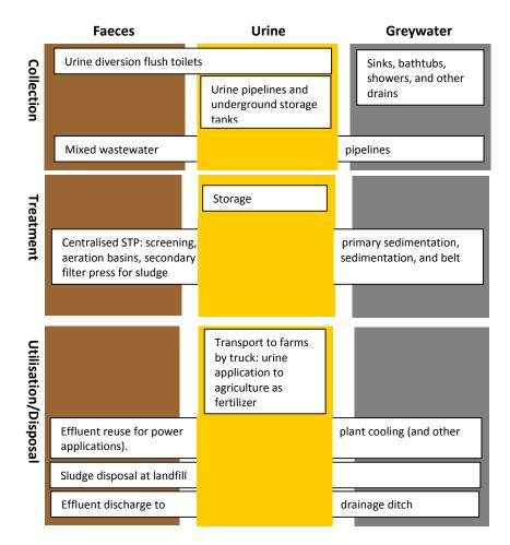
*Figure 9-3.* Alternative DRY System Scenario 2 (Alt-DRY-2) process schematic: Urine diversion with centralized treatment of blackwater and greywater at the Dongsheng STP.
