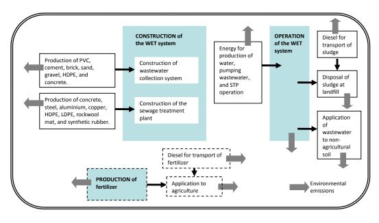
*Figure 5-3.* System boundary for the WET system LCA model. The dashed boxes represent system expansion.
