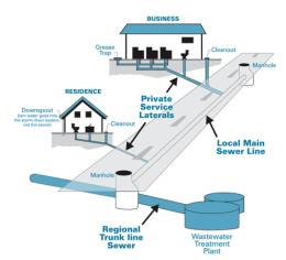
**Figure 7-15.** Illustration of a typical sewer system. The laterals carry one house's or one building's volume of wastewater, local mains carry a sub-area's volume of wastewater, and trunk lines carry a region's volume of wastewater. [Source: http://www.ocwatersheds.com.]
