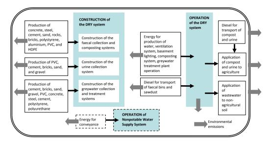
*Figure 5-2.* System boundary for the DRY system LCA model. Environmental emissions for the processes shown were included in the LCA. The dashed boxes represent system expansion.
