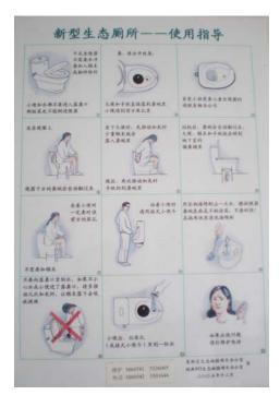
**Figure 7-1.** Instruction poster for the EETP dry toilets. The poster explains how the toilet works, the use of a child-sized seat, the use of the urinals by men, proper cleaning techniques with minimal water, and the O&M support available onsite.
