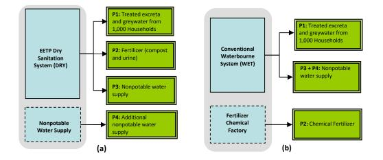
*Figures 5-1a and 1b.* System expansion of the (a) DRY and (b) WET systems as modeled in the LCA.
