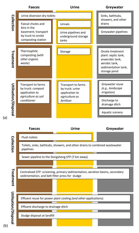
*Figures 3-10a and 3-10b.* The (a) DRY and (b) WET system scenarios and the associated collection, treatment, and utilization/disposal processes. Items in italics had not been fully implemented as of 2009.
