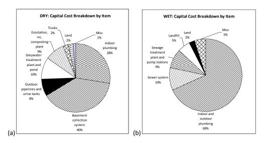
Figures 6-1a and 1b. Capital cost breakdowns by item for the (a) DRY and (b) WET systems.
