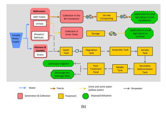
*Figures 3-3a and 3b.* Process schematics of the (a) conventional sewer and centralised Dongsheng STP and (b) EETP dry sanitation system as envisioned (features shown in dashed boxes had not been fully implemented as of 2009).
