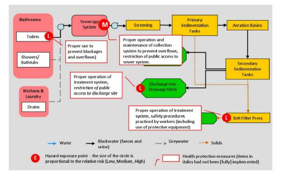
*Figure 7-9.* The hazard exposure points and associated health protection measures to reduce exposure and risk for the WET system.
