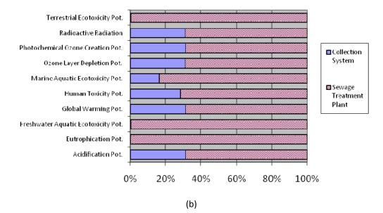
**Figures 5-10a and 10b.** Life Cycle Impacts of the WET system during a) construction and b) operation over a 20-year period broken down by percentage contributions of the system components. Note that system expansion with fertilizer production is not included in these graphs.
