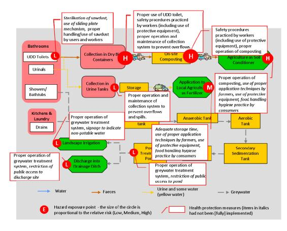
*Figure 7-8.* The hazard exposure points and associated health protection measures to reduce exposure and risk for the DRY system.
