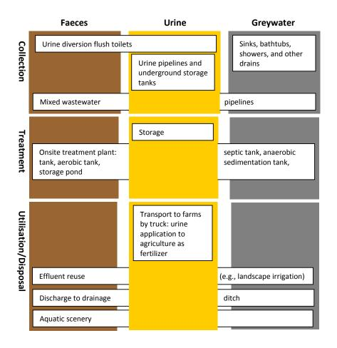
*Figure 9-2.* Alternative DRY System Scenario 1 (Alt-DRY-1) process schematic: Urine diversion with onsite treatment of blackwater and greywater.
