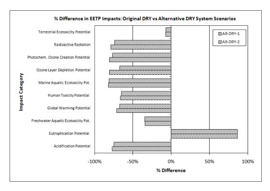
**Figure 9-4.** Results of the Alternative DRY System Scenario Analysis: % Difference in DRY System Impacts. The % Difference was calculated as follows: [(Alternative Scenario Impact – Original DRY System Impact)/Original DRY System Impact x 100%]. Negative % Differences reflect reduced negative environmental impacts, or improved environmental sustainability based on that indicator.
