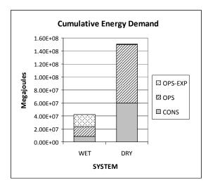
**Figure 5-11.** Cumulative energy demand of the DRY and WET systems broken down by construction, operation, and system expansion.
