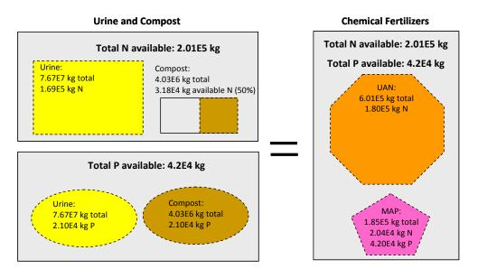
**Figure 5-6.** Components Included in the LCA: WET System – Fertilizer equivalents of urine and compost under system expansion (UAN: Urea- ammonium nitrate and MAP: monoammonium phosphate).
