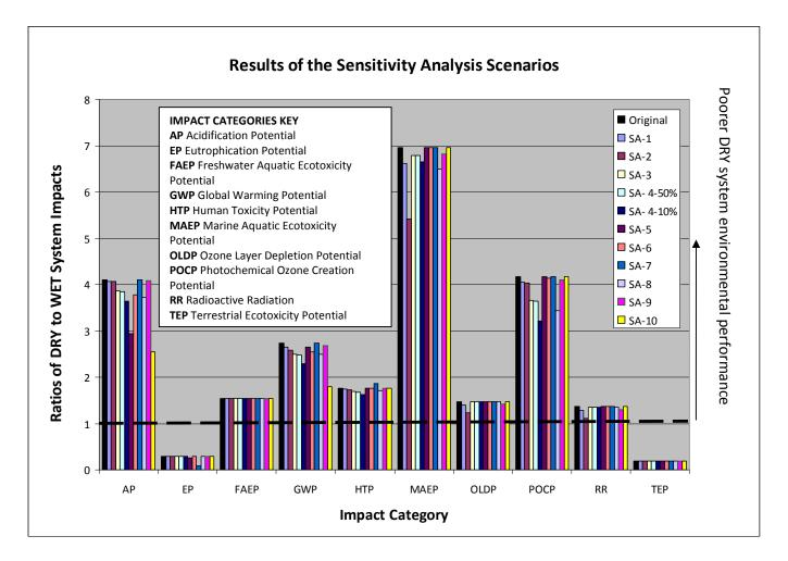
*Figure 5-14.* Normalized ratios (DRY/WET) of the indicator values by environmental impact category under the various sensitivity analysis scenarios. Ratios greater than 1 indicate poorer DRY system environmental performance.
