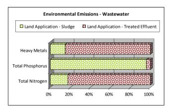
Figure 5-5. Components Included in the LCA: WET System -Environmental emissions of nutrients and heavy metals from domestic wastewater. All emissions are assumed to be discharged to industrial (i.e., non-agricultural) soil.
