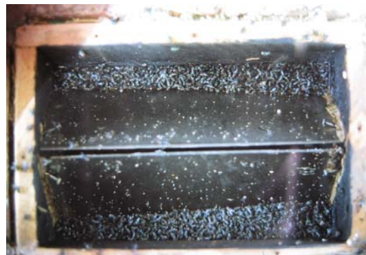
Experimental vent pipe with fly trapping window. Fly trap with flies.
