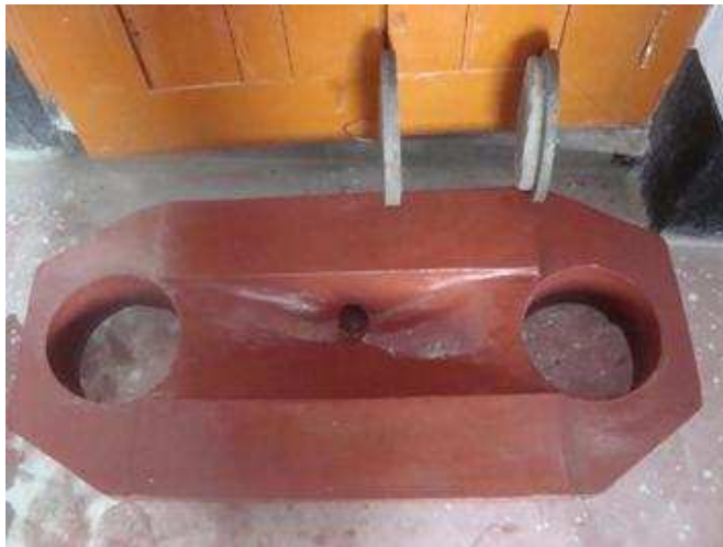
Fig. 7: Completed squatting pan, ready for installation (source: Laxman Kharal Chetty, 2009)
