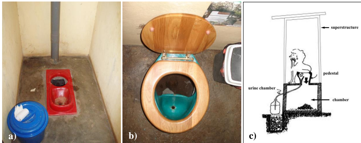
Figure 9: Source separating toilets. Picture a) shows a urine diverting dry squatting pan (Uganda), b) a western style urine diversion dehydration toilet (UDDT) (Mexico) and c) a sketch of a UDDT (own photographs and Esrey et al. 2001).
