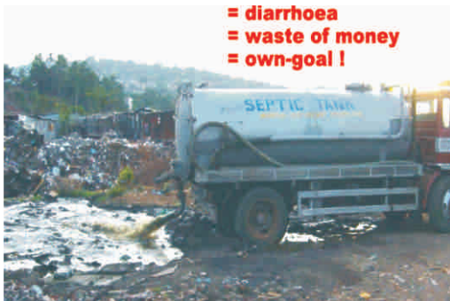
Figure 39 : Sadly typical means of waste disposal, often into streams and wasteland
