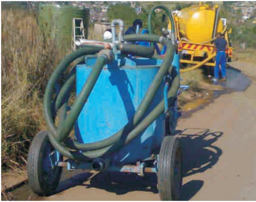
Figure 30 : Vacutug being trialled in Pietermaritzburg
