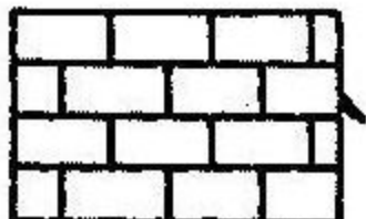
Stretcher bond: one-brick wall
