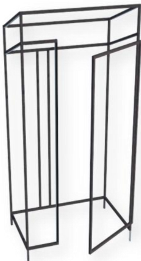
Latrine shelter frame
