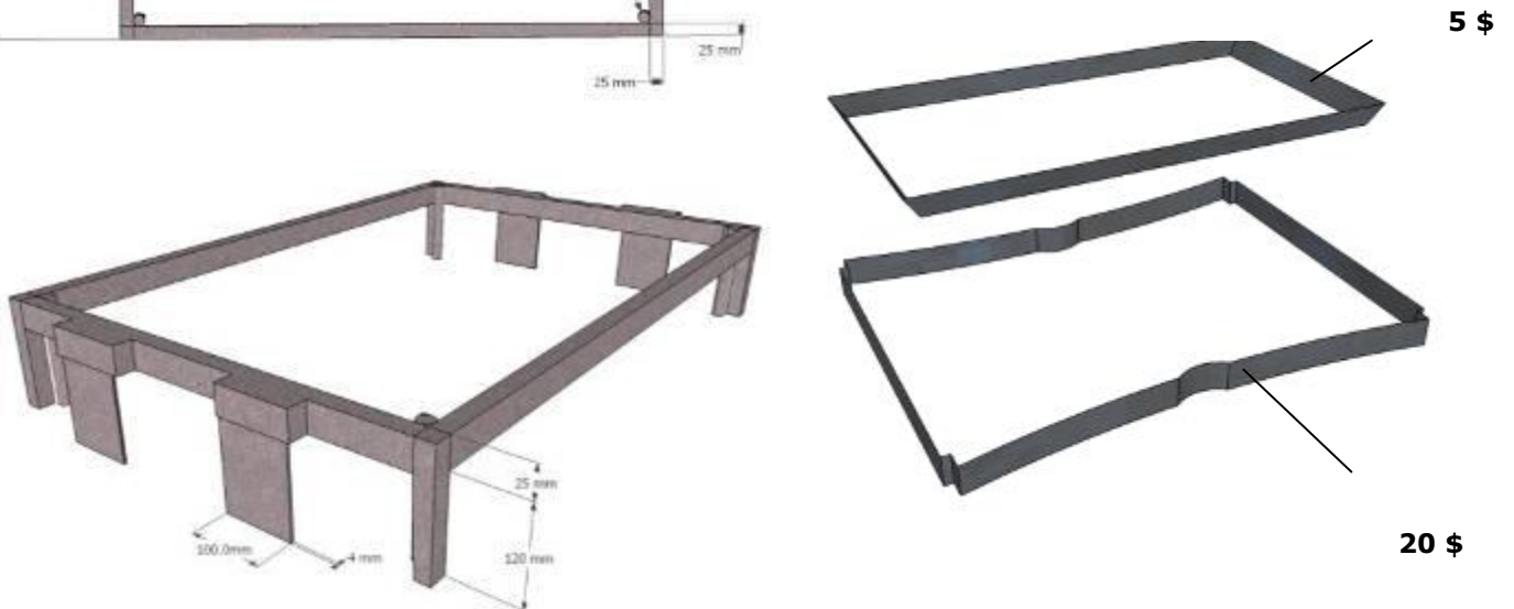
Molds for Slab
