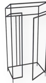
Latrine shelter frame
