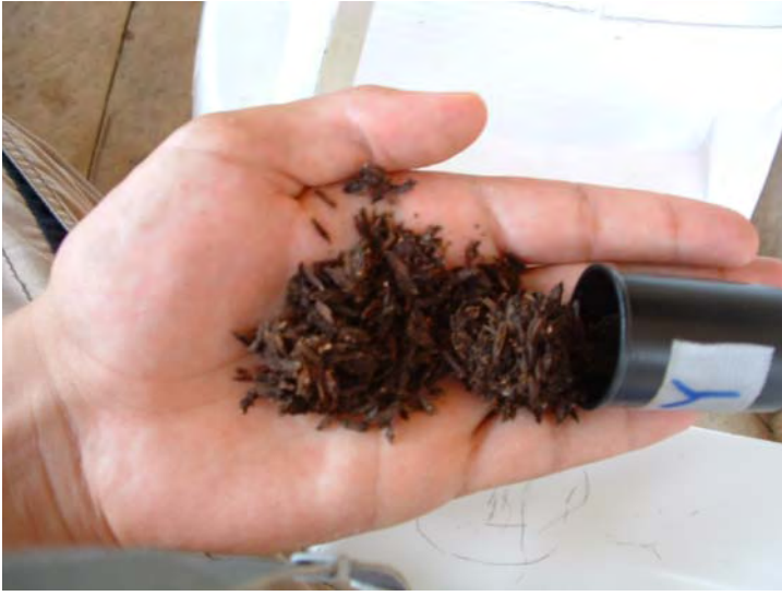
Figure 27. A sample of matured compost taken from the author's composting latrine in Kusapin, Panama. Note the humus-like appearance. The compost had no distinct odor.
