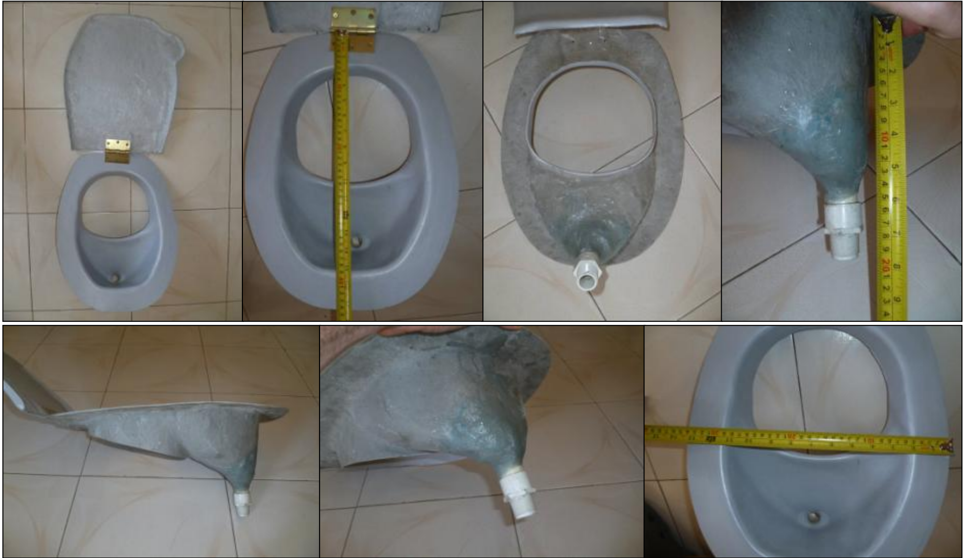
PHOTO T15: SOIL UD Toilet seat from fibreglass
