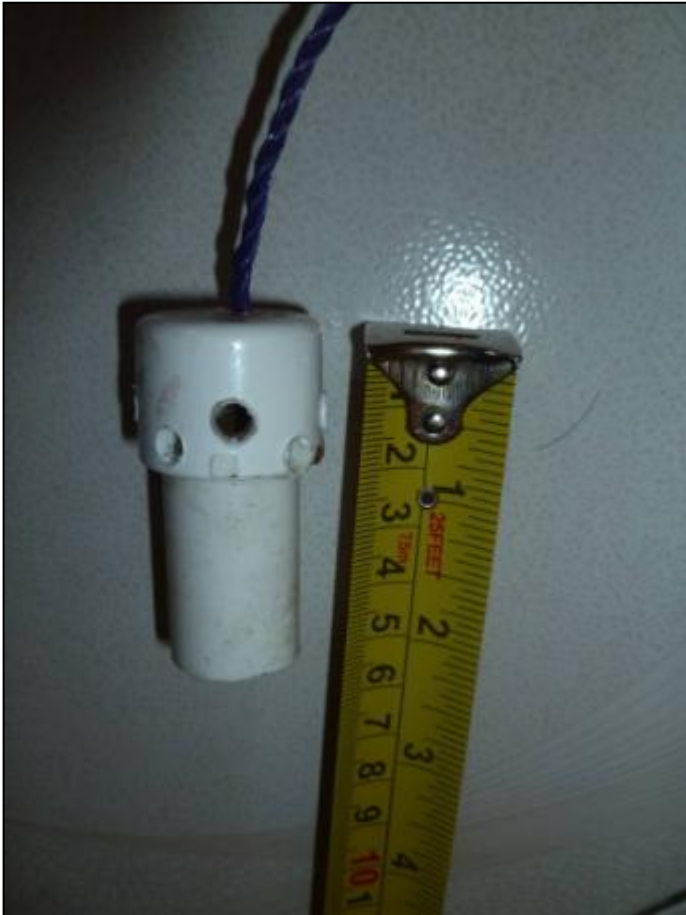
PHOTO T14a: PVC filter with security cord attached
