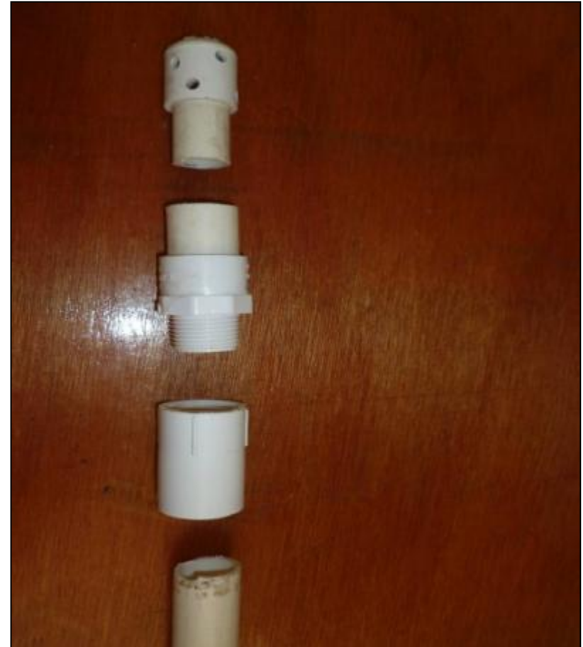
PHOTO T14b: PVC pipe fittings for SOIL UD toilet seat
