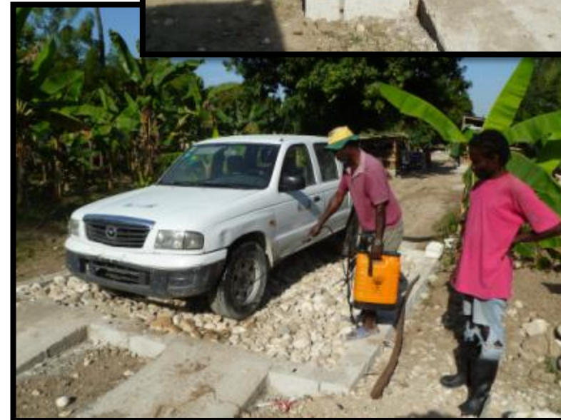
Photo K218a,b: Chlorine spray station for vehicles
