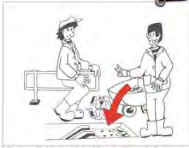
The operator disposes of the debris together with the screenings removed at the inlet works. It is allowed to drain before disposal in an excavated trench (see page 8)
