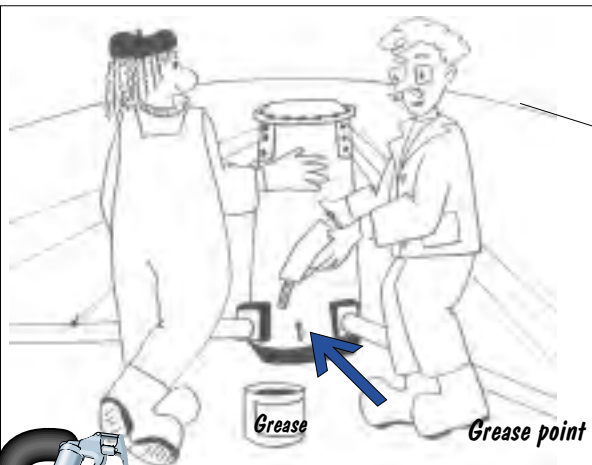
The operator and supervisor lubricate the centre column at all the designated grease points
