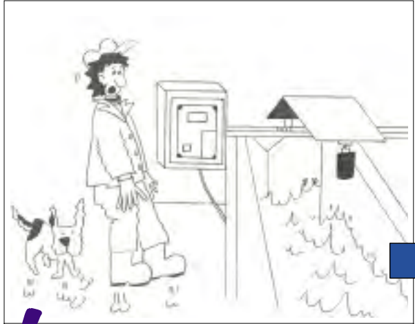
! The operator checks on the flow regularly. Turbulence causes incorrect readings
