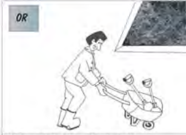
If there are no desludging valves, the pond is decommissioned and the sludge is allowed to dry. The operator can now remove the sludge with a spade and wheelbarrow
