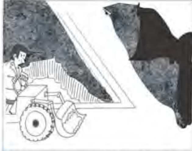
OR The operator can also remove the dried sludge with a front loader, if available
