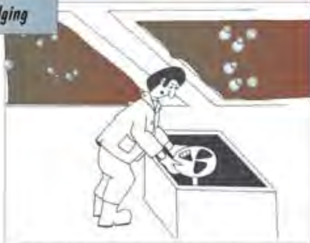
The operator opens the desludge valve when excessive rising bubbles are observed in the waste water in the ponds
