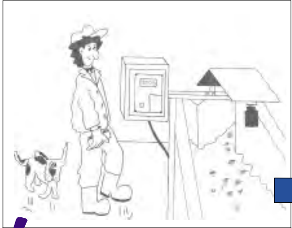
! Grit that has been washed out or not removed from the grit channels may cause incorrect flow meter readings
