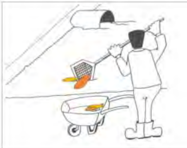
The operator removes floating debris from the surface
