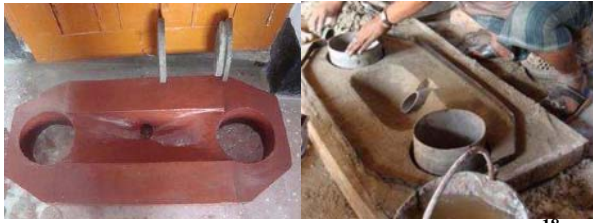
Figure 21: UDDT Double Vault Squat Pan 18
