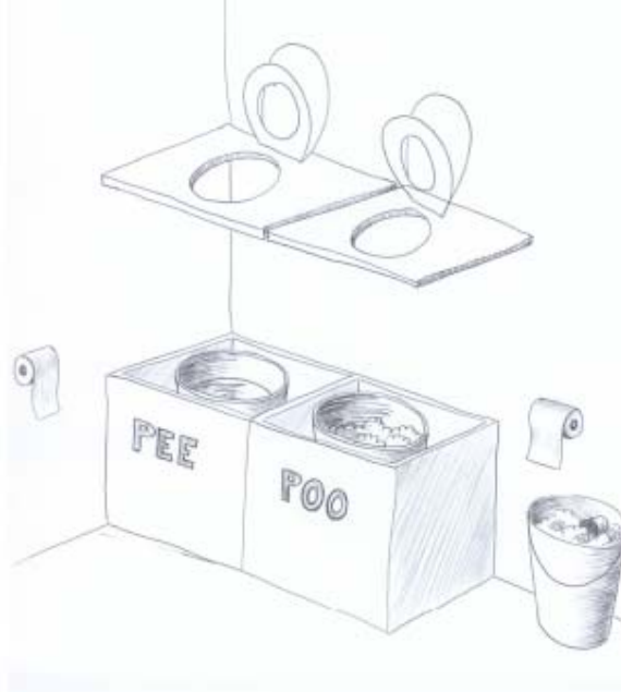
Figure 26: Emergency Composting Toilets in New Zealand 23
