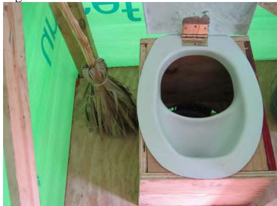
Figure 19: UD toilet seat developed by SOIL and manufactured in Port-au-Prince. 17
