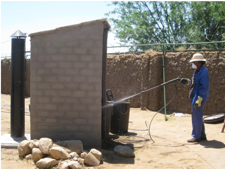
Picture 6: Washing bins for reuse at CHP. Emptied bins are cleaned in a construction for this purpose at CHP. Beneficiaries of Otji-Toilets in Otjiwarongo are provided with washed bins after the cleanout. Source: Picture taken by authors.
