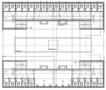
**Fig. 7:** Floor plan of the UDDT block. Top: female section with 15 cubicles; Bottom: male section with 9 cubicles and 6 urinals in the middle (source: GTZ-IS, 2008).
