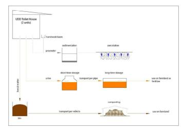
Fig. 4: Design of the UDDT system and treatment steps (source: Oldenburg et al. (2009).
