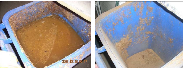
Figures 5a and 5b. A bin resulting from improper use, i.e. user is discharging excessive water into the faecal chute (left). A bin from a properly-used dry toilet (right).
