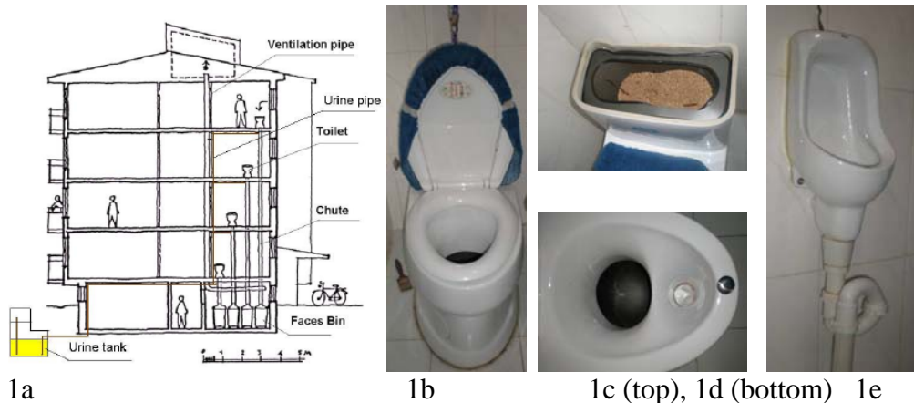
Figures 1a-e. The EETP and its dry toilets and urinals. 1a. A schematic of an EETP multi-storey building illustrating how the toilets are connected to the faecal collection bins in the basement and urine storage tanks (from Zhu, 2008). 1b. A UDD toilet. 1c. The sawdust dispenser of the UDD toilet. 1d. The UDD toilet with the faecal hole in the back (left) and the urine hole in the front (right). The metal button in front turns the faecal collection bowl upright when activated by the user's weight; when the user stands up, the bowl turns 180° and releases the bowl contents into the chute. 1e. Waterless urinal.
