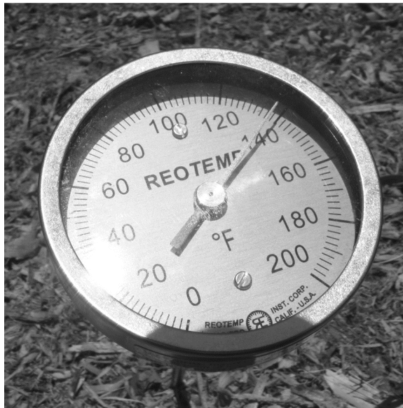
Figure 8: Temperatures recorded in Haiti's humanure compost piles ranged from approximately 46C to over 70C. This is approximately 60C. Fluctuations vary according to size of pile, age and contents.
