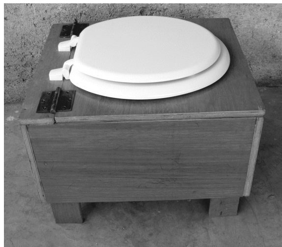
Figure 1: Typical 20 liter capacity humanure toilet in Haiti.
