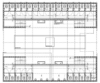
Fig. 5: The floor plan of the UDDTs complex. Top: female section; Bottom: male section (Source: GTZ-IS (2008)
