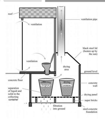
**Fig. 5:** Functional plan of the Otji toilet without urine diversion bowl as shown in Fig. 4 which was developed later (source: CHP, 2009b)
