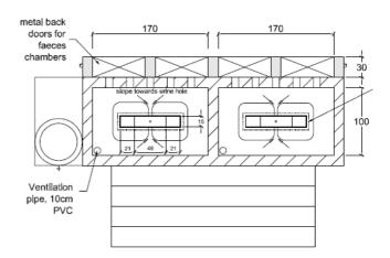
**Fig. 9** Top view of toilet block with 2 UDDT cubicles and hand washing unit (source: Rieck, GTZ, January 2010)
