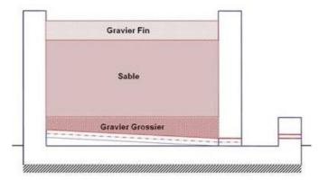
Fig. 6: Profile of the filter with the different layers (source: AHT, 2011)
