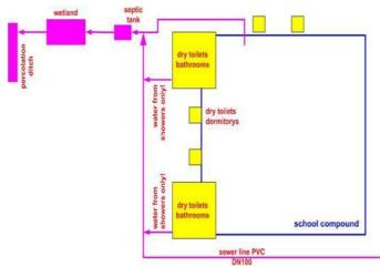
**Fig. 7:** Scheme of new greywater system; flow is from right to left (source: EcoSan Club).
