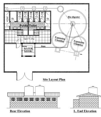
**Fig. 9:** Technical drawing of the facility and biogas plant (source: EPP). Space requirement for toilet and biogas plant is approx. 10 x 15 m.
