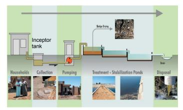
**Fig. 6:** Schematic of the rural sanitation system, with a Small Bore Sewer System connected to a pond system for treatment (source: GIZ; 2006).
