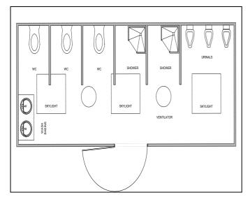
Figure 6: Typical design of a CAB (source: EWS, 2009).
