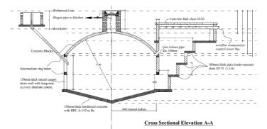
**Fig. 10:** Technical drawing of the biogas plant (built completely underground). Diameter of dome-shaped digester is 5 m. See section 13 for links to further drawings (source: EPP).
