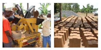
**Fig. 14:** Left: Production of hydraform blocks; Right: completed hydraform blocks (Source: Paul Mboya, June 2009).
