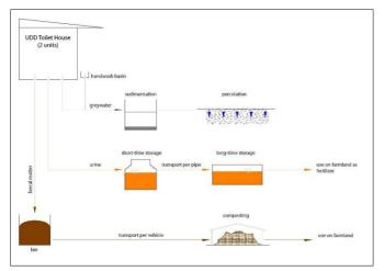
**Fig. 4:** Design of the UDDT system (source: Oldenburg et al. (2009)).
