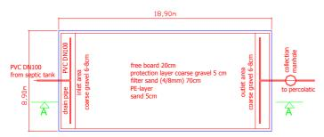
**Fig. 9:** Plan view of horizontal flow constructed wetland, flow is from left to right (source: EcoSan Club).
