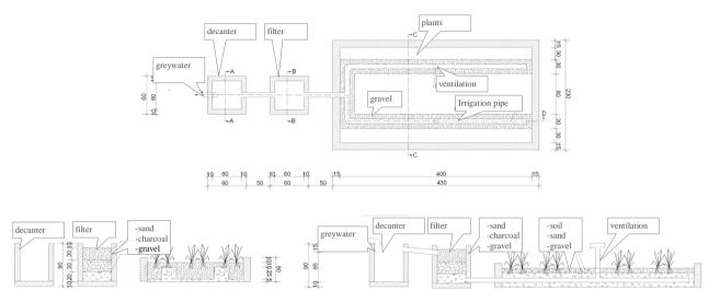
Fig. 11: Plan view and cross sections of the greywater garden (source: OtterWasser, 2003)
