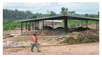
**Fig. 3:** Co-composting facility (open windrow system) in Kumasi (source: IWMI, 2003).
