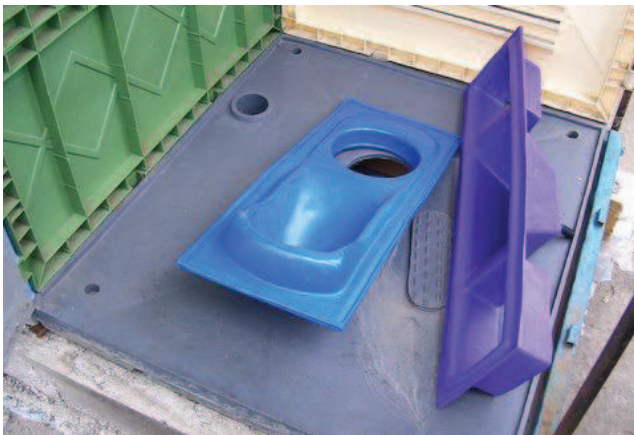
Fig. 10: Various urine diversion plates at the factory of Kentainer. The double vault plate was developed by EPP (source: C.Rieck, GTZ-Kenya, Jan 2010).
