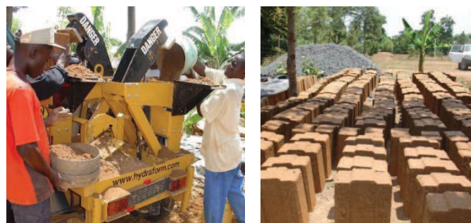
Fig. 14: Left: Production of hydraform blocks; Right: completed hydraform blocks (Source: Paul Mboya, June 2009).
