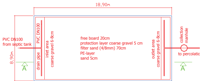
Fig. 9: Plan view of horizontal flow constructed wetland, flow is from left to right (source: EcoSan Club).
