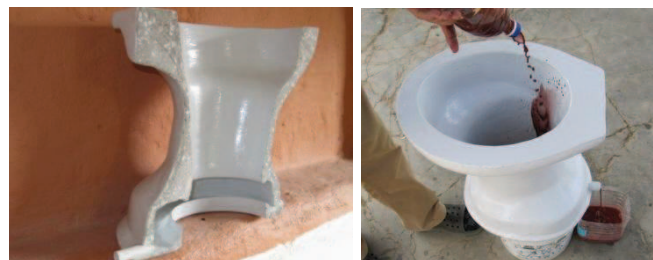
Fig. 4: Cross section of the new urine diversion bowl (left) made from painted concrete where urine collects in the little trough at the bottom as demonstrated in urine diversion bowl (right) (source: CHP, 2009a).
