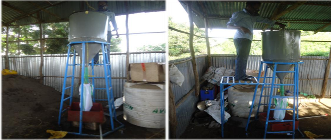
Figure 3 - Photos taken during the mixing of the solution (stored urine plus MgO)
