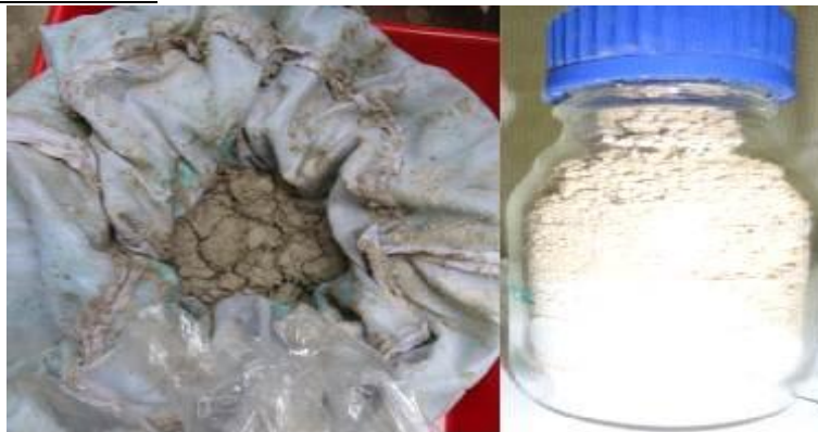
Figure 9 - Struvite precipitate exposed to sun light and dried struvite in a glass bottle
