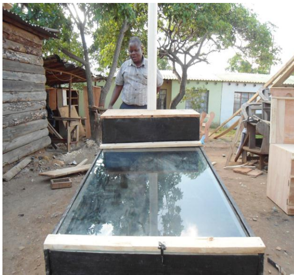
Fig 1: A solar Sludge Drier ready for testing
