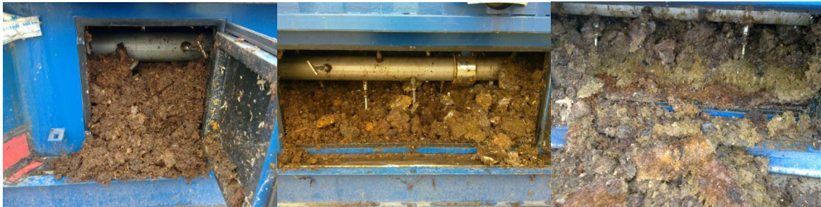
Figure 3: The quality of faecal sludge from the different toilets of the MobiSan
