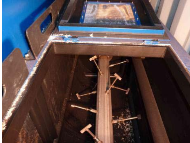
Figure 2: Faeces chamber (with separation channel – Mels et al., 2008)
