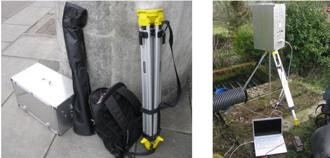
Figure 1: The portable penetrometer packed for transport and in use testing a septic tank
