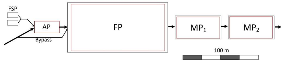
Figure 5.10 – Design and size of WSPs (black: Site A, red: Site B)
