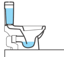
Figure 2.4 – Flush toilet (Tilley et al., 2008)
