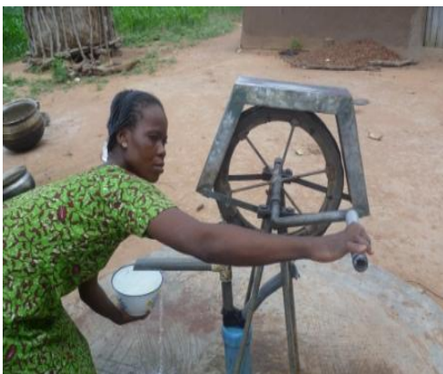
Figure 6. New Rope Pump design
