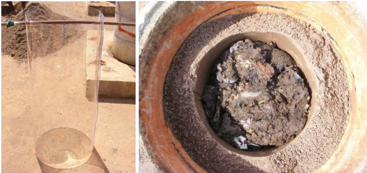
Figure 5.60 A polycarbonate cylinder (left) was used to fill the tower with a core of sludge ringed by river sand (right)
