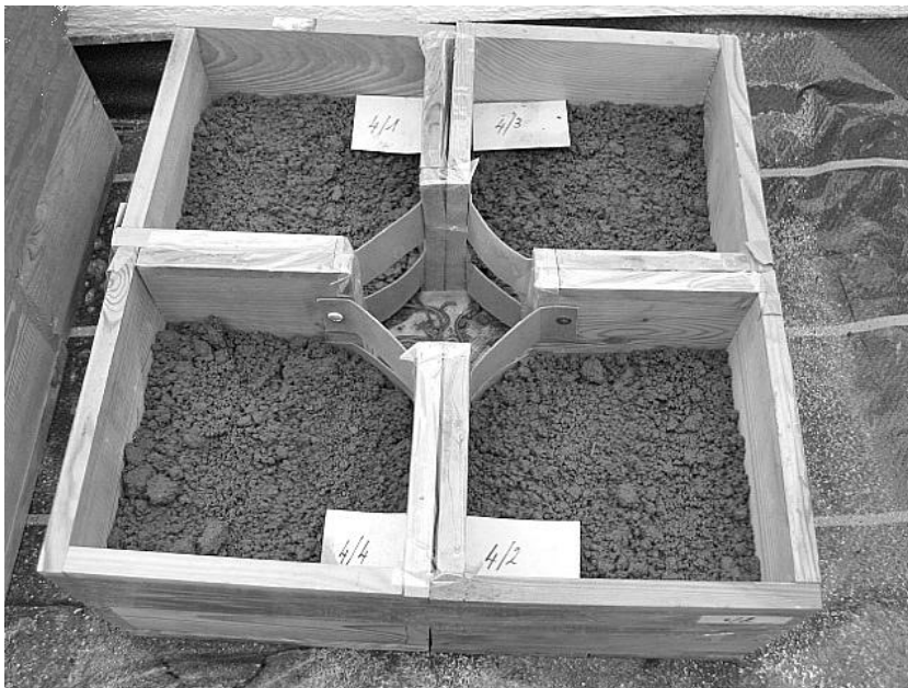
Figure 9: Wooden boxes used for Avoidance Response Tests, worms placed in the middle
