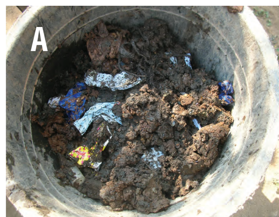
FIGURE 2 (a) Dry sludge removed from pit; (b) Solid sludge and non-faecal matter prevents measuring stick reaching bottom of pit
