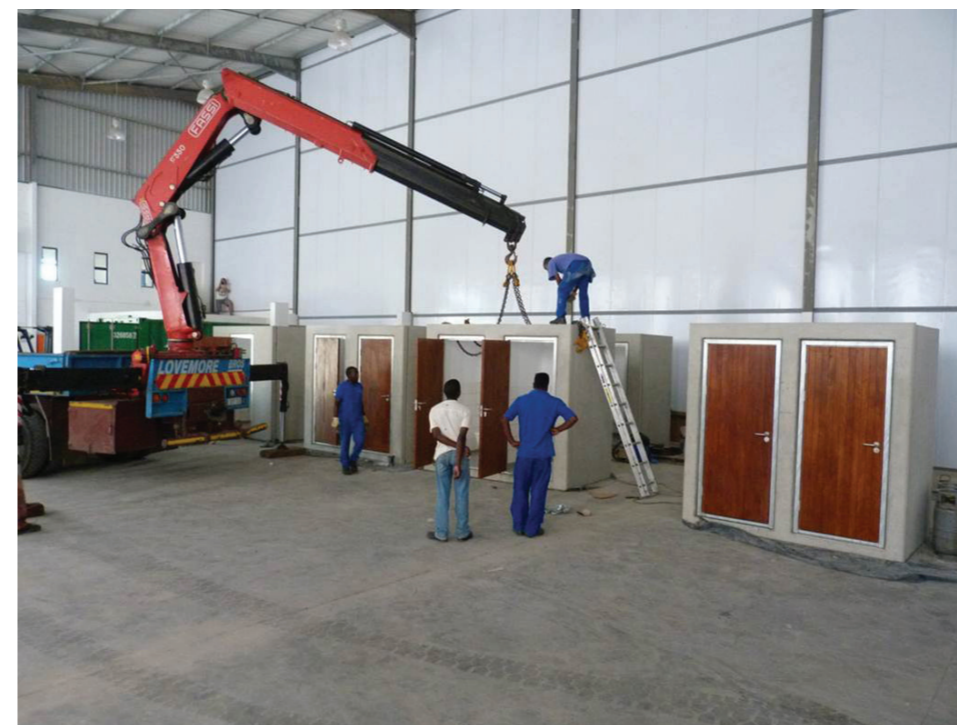
FIGURE 2 Manufacturing toilet modules in a factory
