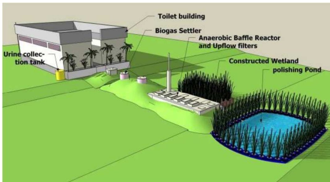
Figure 6.7 School toilet block with pour flush and urine diversion in Badlapur, India (Panesar and Bischoff, 2008)
