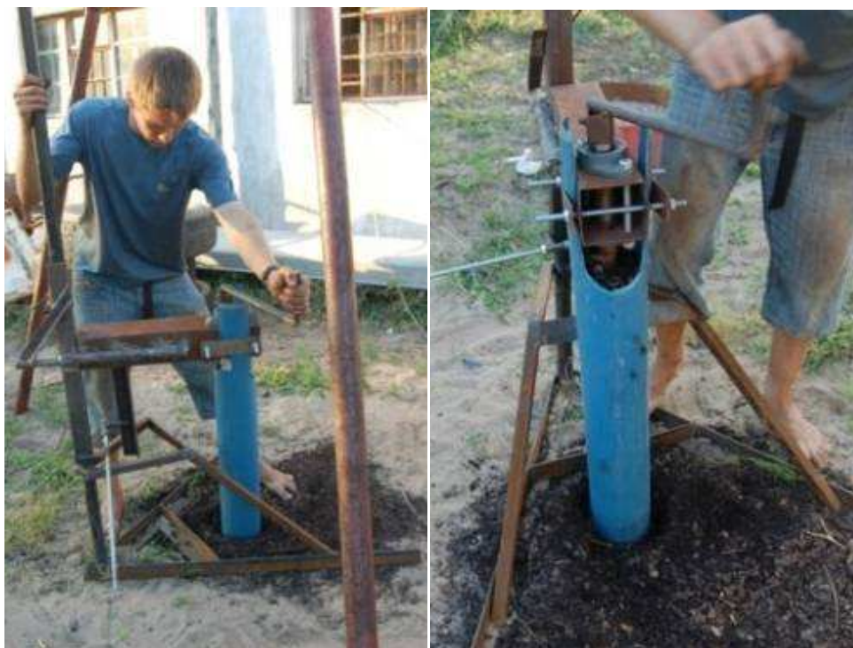
Figure 4.30 Prototype of manual pit screw auger (O’Riordan)
