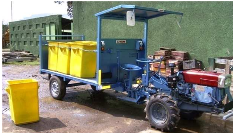
Figure 5.2 Chinese two-wheeled tractor used for solid waste collection (UN-HABITAT)
