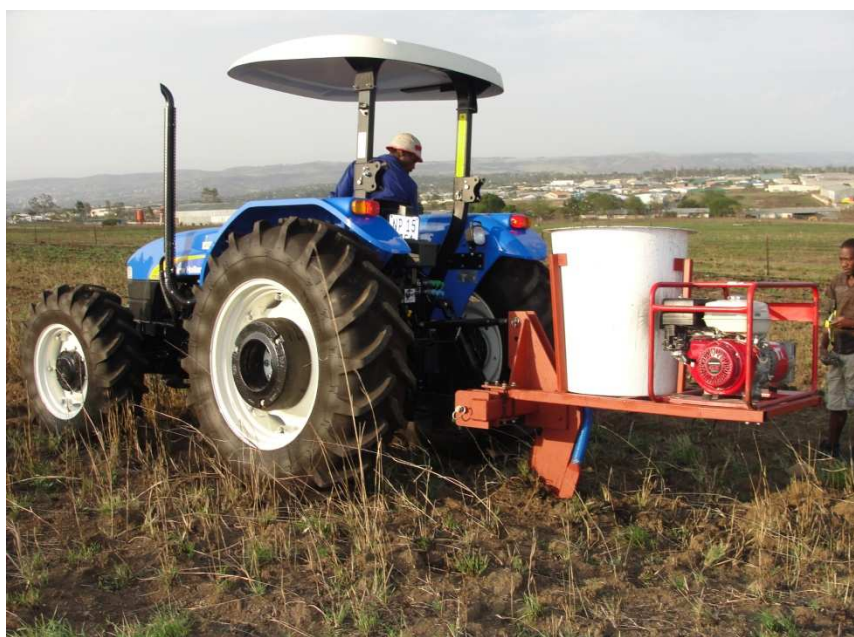
Figure 6.21 Field testing the sludge injector
