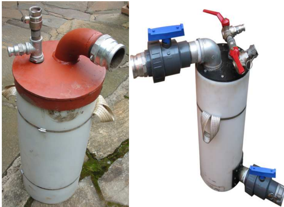
Figure 4.36 The “suck only” arrangement (left) where a removable lid is used for multiple vessels and the “suck and blow” arrangement (right) which uses a single vessel and lid
