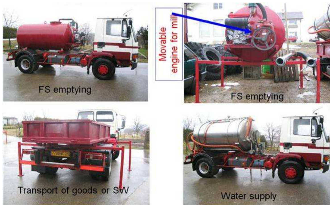
Figure 5.6 A single truck which can be adapted for either refuse collection, or water delivery or vacuuming (Eawag and Sandec)
