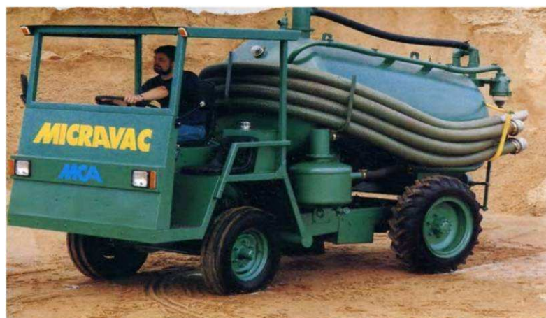
Figure 4.24 Micravac latrine emptying vehicle (Coffey)
