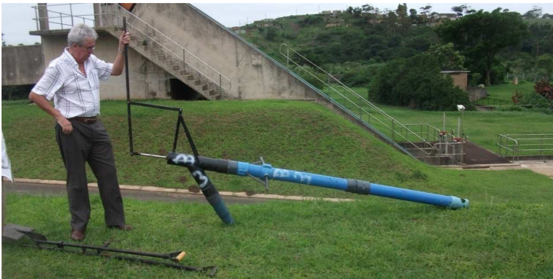
Figure 4.11 The Modified Gulper, with lever action added
