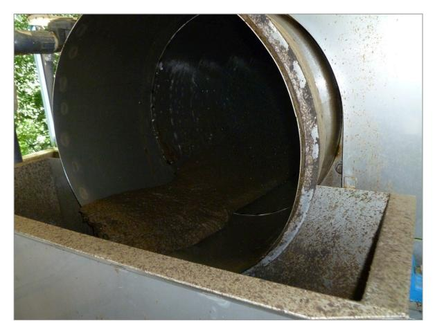
FIGURE 3: Discharged thickened sludge
