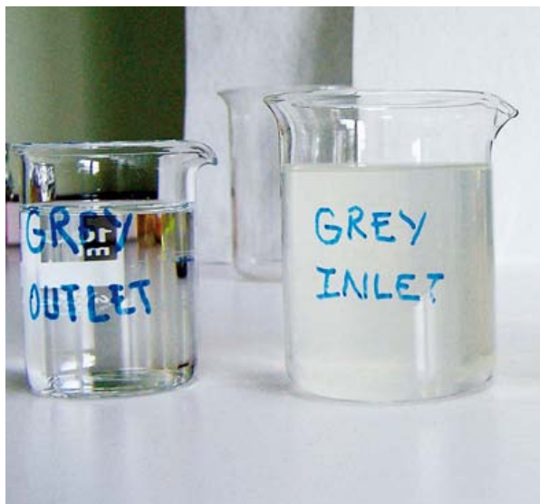
► Figure 6: RAW GREYWATER AND EFFLUENT OF THE MBR
