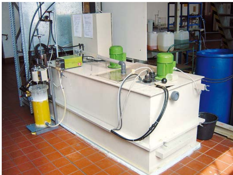
▲ Figure 5: 500 L PILOT SCALE SM-SBR FOR THE TREATMENT OF GREYWATER AT THE TECHNISCHE UNIVERSITÄT BERLIN, GERMANY
