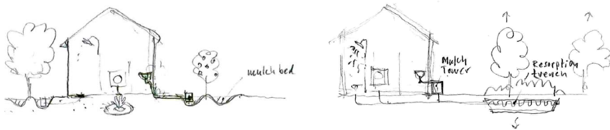
Figure 19. Greywater treatment with mulch. Direct single-source treatment in mulch basins (left); joint-source treatment in mulch tower and irrigation of respiration trench (right). (Sketches: Peter Ridderstolpe)
