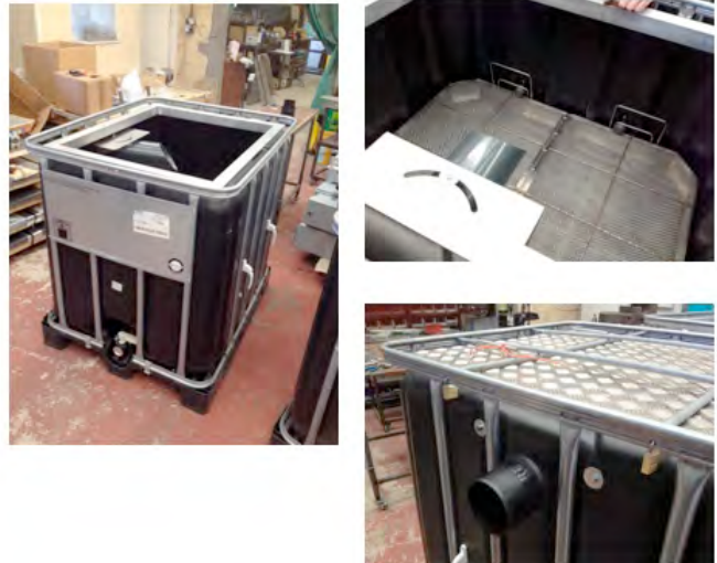
Figure 10 - Modified IBC with customised internal worm baskets, waste-in deflector and security lid
