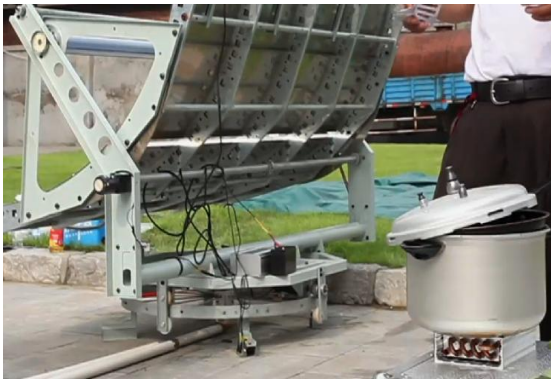
Solar collector used to power hotplate for cooking or water purification
