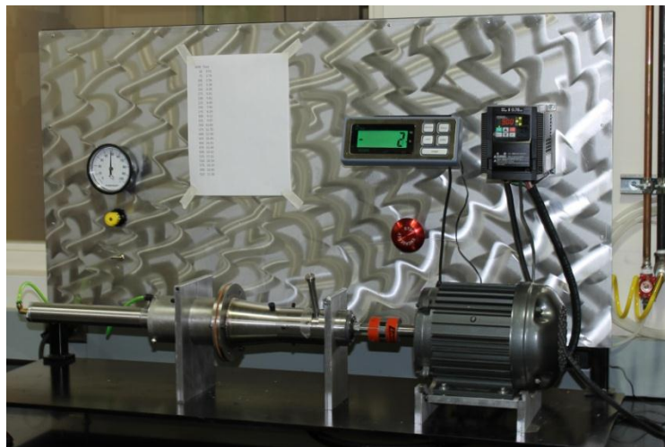
Figure 4. Instrumented reactor to process faecal and simulant solids
