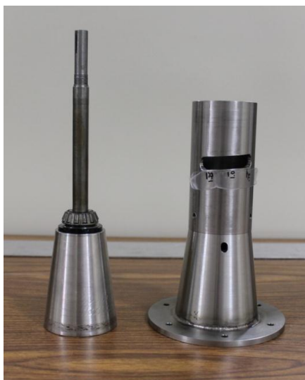
Figure 5. The cone (left) rotates inside the housing (right).
