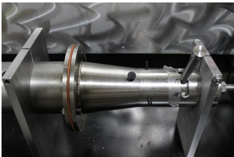
Figure 6. A typical setup of the cone inside the housing with spacing controller and outlet corked (black)
