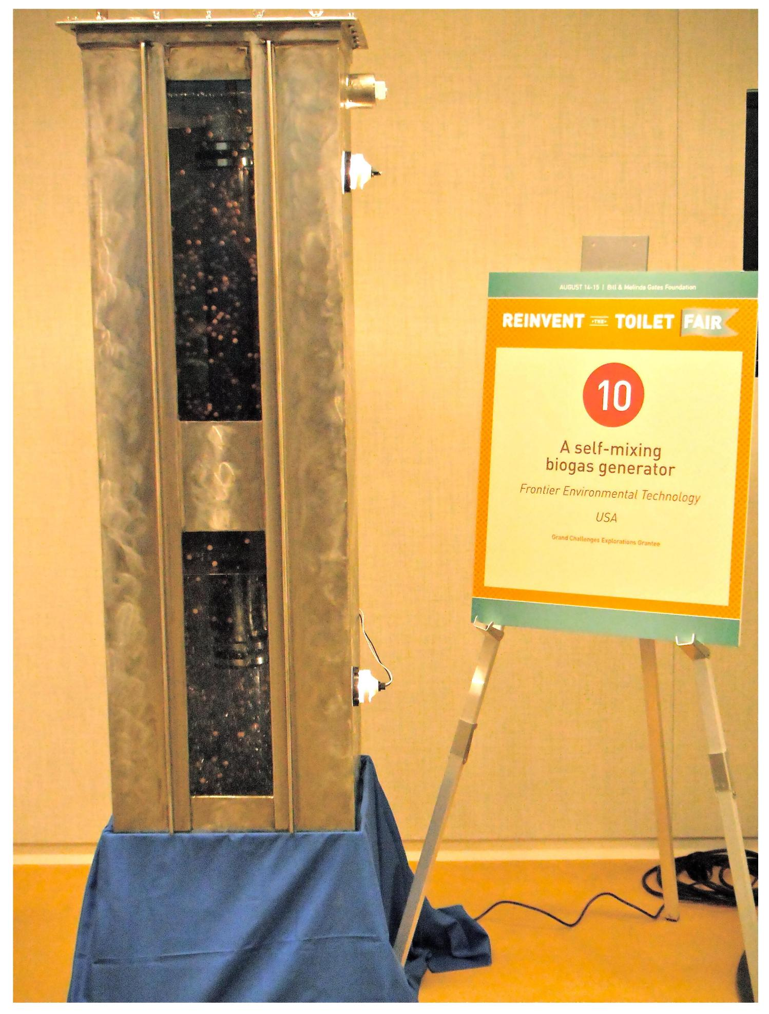
The prototype Self-Mixing Biogas Generator on display at the Reinvent the Toilet Fair represents the size of the reactor needed to treat waste from one individual at  $20^{\circ}$  C – approximately 60 gallons. If the temperature of the reactor is raised to 35° C the same size reactor can treat waste from two individuals. The temperature of the reactor in the field could be raised by passive solar heating while installation below grade provides insulation at night.
