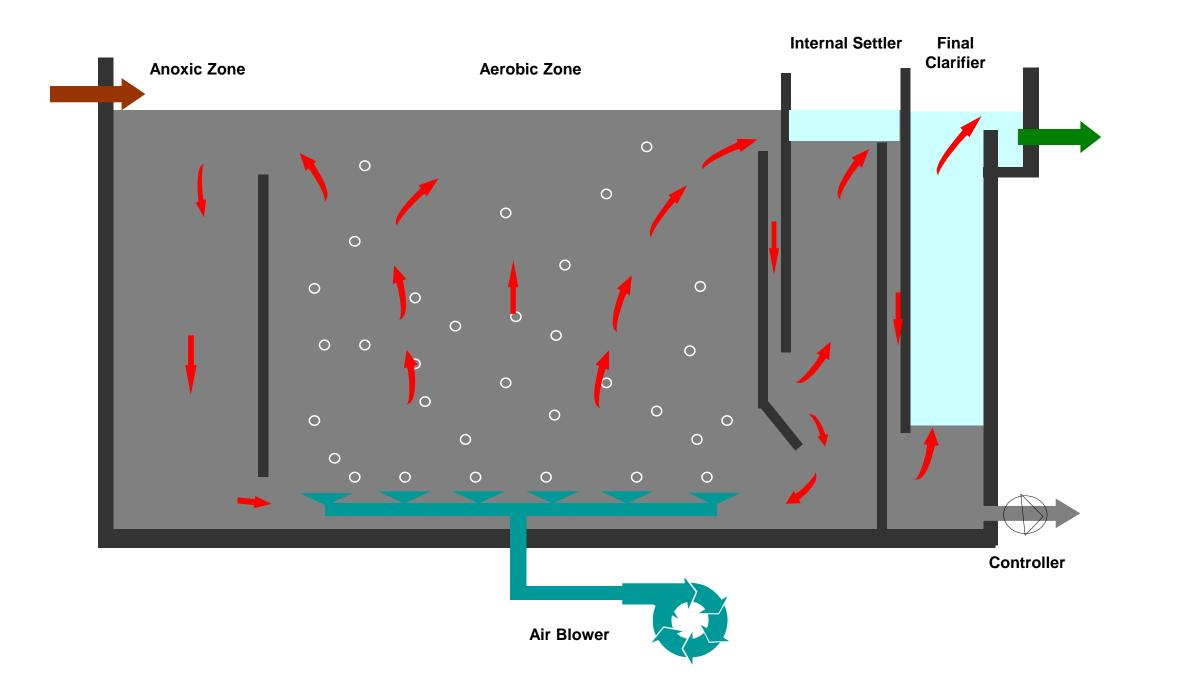
• Surge Pumps – Modified airlift pumps designed to mix and transport fluid using large-diameter bubbles that minimize oxygen transport to the fluid. These pumps provide reduced operational costs over conventional means of mixing and transport. The Surge Pump represents the key innovation of the Self-Mixing Biogas Generator.
