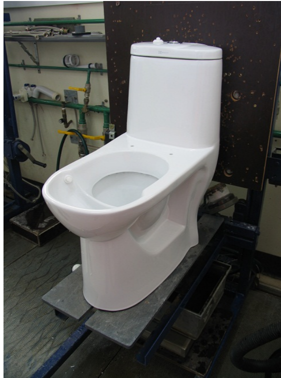
Figure 43: UDT performance being tested on NATA laboratory test rig.
