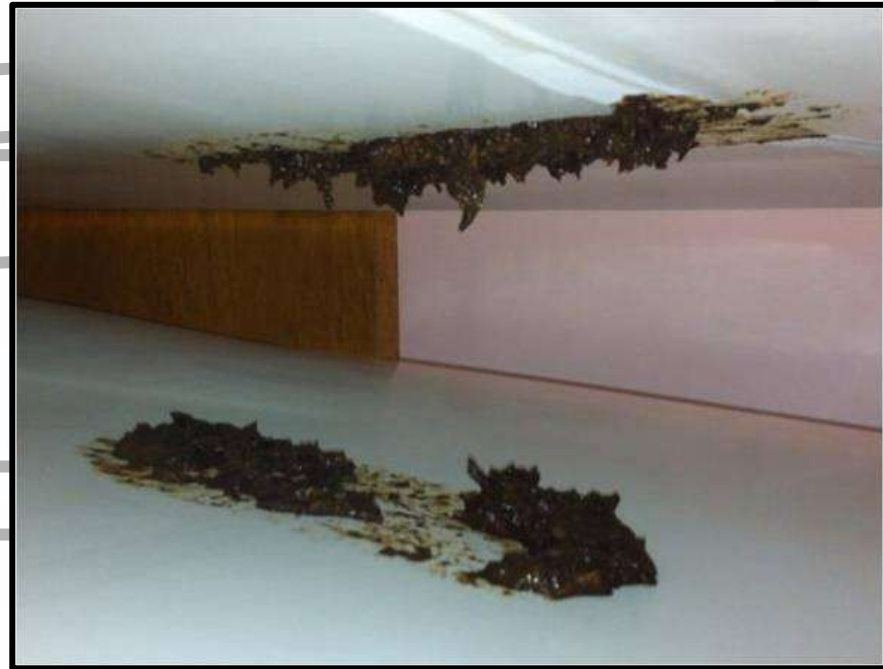
Flattened feces splitting on top & bottom belt
