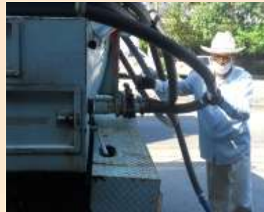
(c) Turn on vacuum pump
