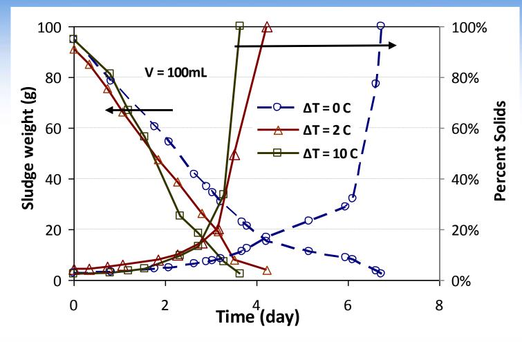
Greater  $\Delta T$  speeds up drying, but 2C difference seems sufficient
