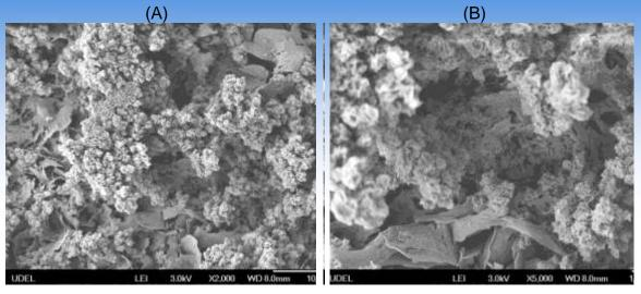
SEM images of PVDF membrane surface (A) and (B) and cross section (C) and (D) after 1200 hours DCMD of instant ocean salt.
