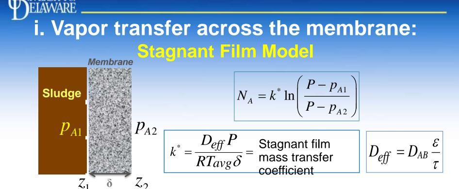
$N_{A} = \text{flux of water across membrane (mol \cdot m^{-2} \cdot s^{-1})}$  P = total pressure of water vapor and air (Pa)  $p_{A2} = \text{partial pressure of water vapor on feed side (Pa)}$   $p_{A2} = \text{partial pressure of water vapor on exit side (Pa)}$   $D_{AB} = \text{diffusivity of water vaport in air (m^{2} \cdot s)}$   $D_{eff} = \text{effective diffusion constant (m^{2} \cdot s)}$
