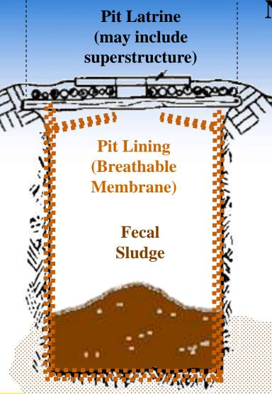
Non-piped toilet equipped with membrane distillation system
