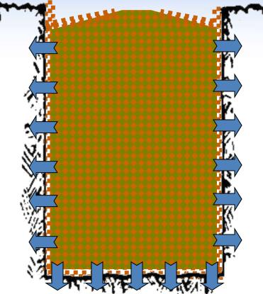
Drying rates now known for sludge/membrane/air: assume this applies unsaturated soil
