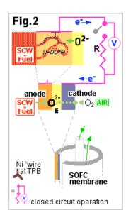
The tSOFC is composed of three strongly bonded but structurally and functionally distinct concentric cylindrical ceramic layers.
