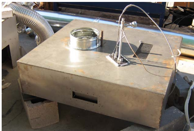
Figure 16. Assembled pyrolysis / combustion chambers.
