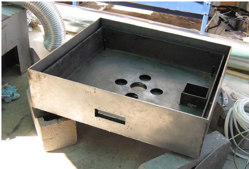
Figure 6. The combustion region of the pyrolyzer featuring a central hole for injecting warmup gas, while the surrounding four holes provide warmed incoming air from the heat exchangers for the lean-burn combustion.
