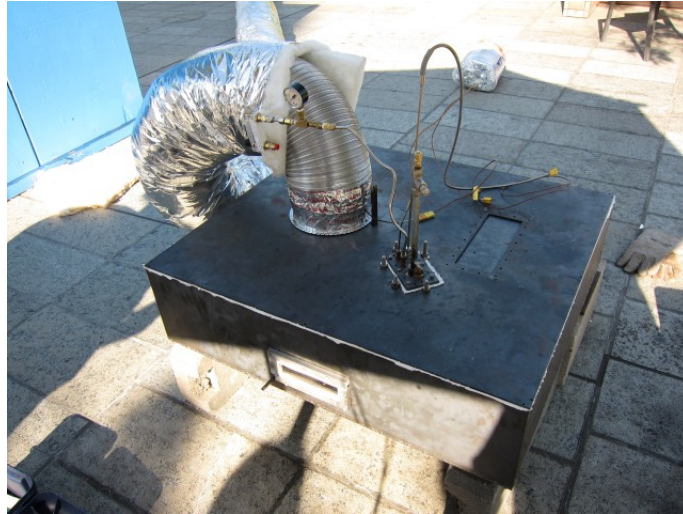
Figure 13. The heat exchanger attached to the top of the reactor.
