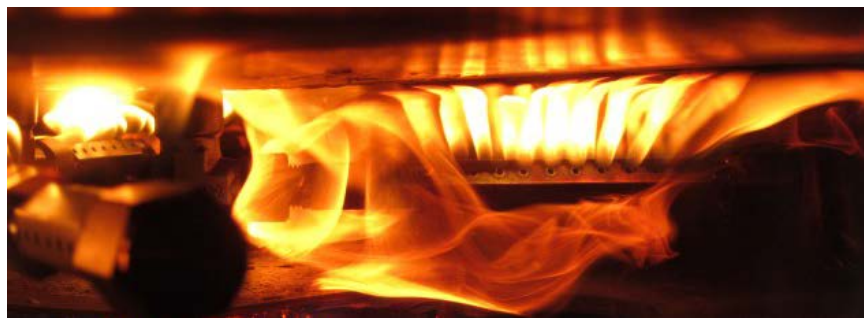
Figure 9. Syngas being combusted in the lean-burn chamber.
