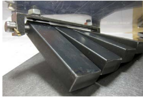
Figure 10. In the prototype, one scraper assembly consists of four leaves.
