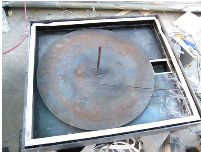
Figure 15. A top view of the rotating turntable and turntable shaft placed inside the pyrolysis chamber.
