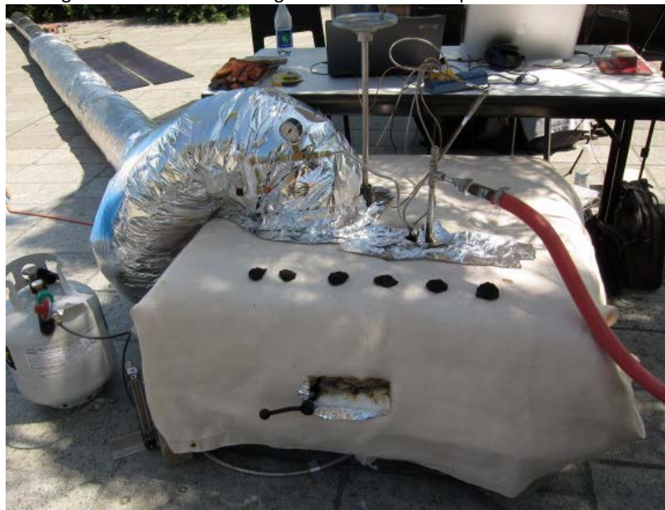
Figure 14. Insulated reactor and heat exchanger, with HSW input feed (red tube).
