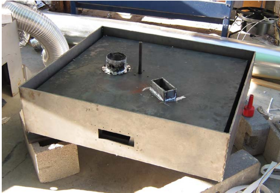
Figure 7. Gas exhaust and HSW input ports on top of the combustion (second) shell. The view is rotated from the view in Figure 5.
