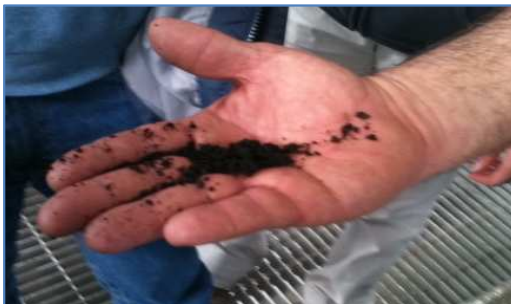
Figure 18: Pelletized biosolids Pellets reach 65%-70% solids composition
