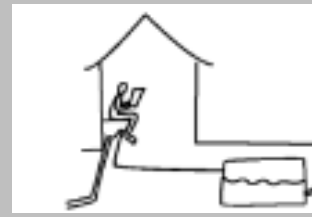
Septic tanks for excreta
