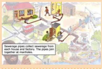
Black/ grey water collected through sewerage network
